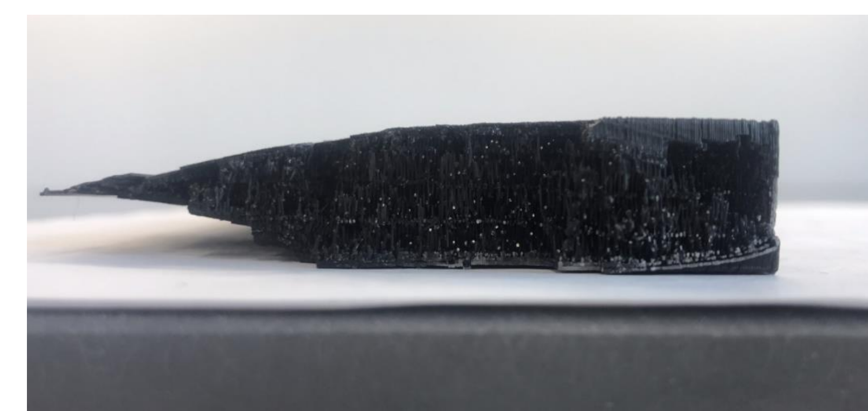
Fig. 8 Side View of Smooth Sample (After Testing) (Failure Mode: Fiber breakage) Adapted from Dongyang Cao
