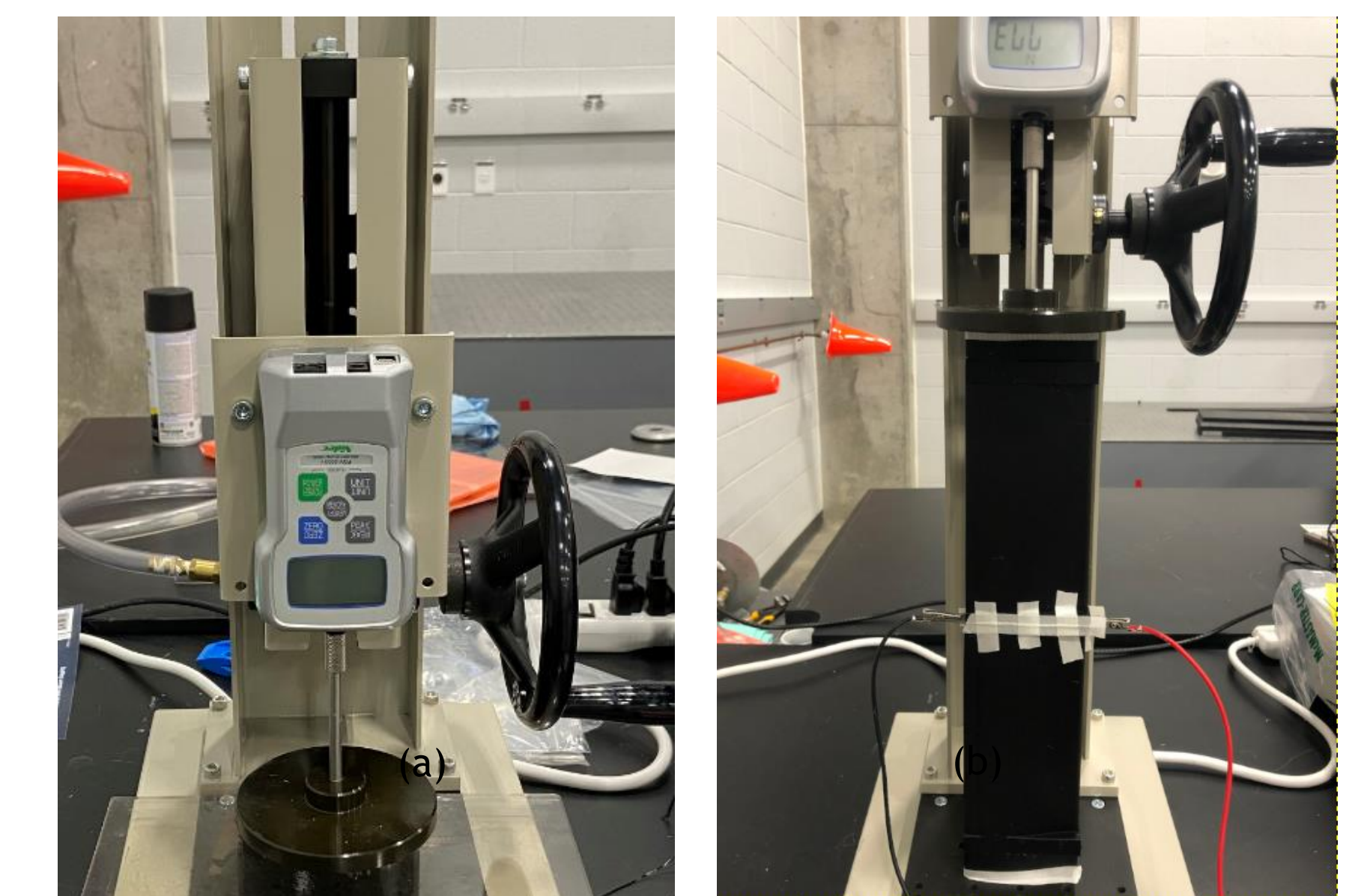
Fig. 9 (a) Resistance welding setup without sample inserted (b) Resistance welding setup with sample inserted Adapted from Dongyang Cao
